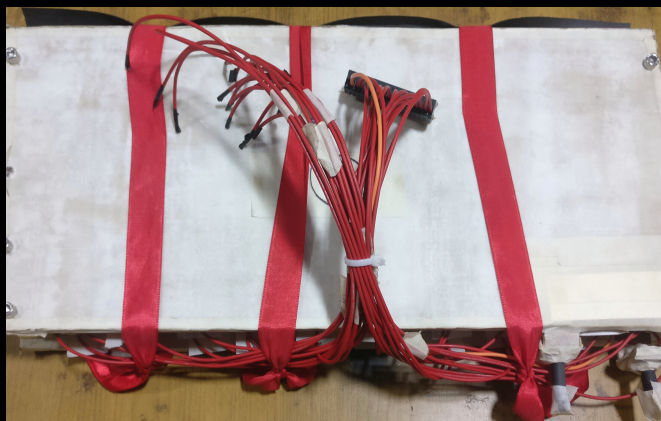
An accumulator segment is shown with the cell tabs and the thermistor connections attached.
